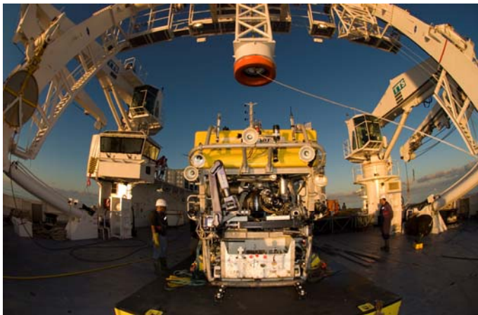
Fig. 2: Victor 6000 on the deck of the oceanographic vessel Pourquoi pas? MoMARETO 2006 © Ifremer
