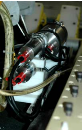
Fig. 12: Methane sensors installed in Victor 6000's survey module (left). They are in line with the newly developed water sampler PEPITO allowing a direct comparison of sensor signals and water sample methane measurements. Right: The power supply of the autonomous methane module.
