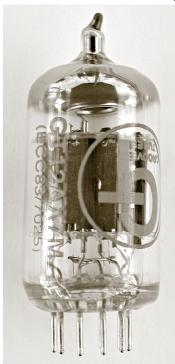
was heralded as the first twin-triode device engineered for high gain, low noise applications and its high voltage gain made it popular with tube amplifier enthusiasts.
