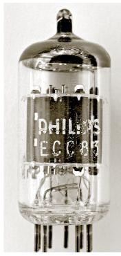
12AX7s manufactured after the mid 1950's feature improved construction with the helically wound heater invented by Sylvania by Gehrke, Huntington, and Granger. Their patent (US2677782-A 2,867,032) highlights longer tube life as major benefit of the invention, however the helical heater also minimizes AC heater supply noise in the tube's output.
