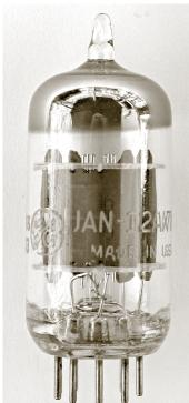
just a model number, it contains quite a bit of information about the tube. The '12' indicates that the heater (the part that glows orange when the tube is powered up) requires 12 volts to operate; the 'A' indicates the tube is an amplifying component; the 'X' identifies the tube's electrical characteristics, that is the gain factor, plate (anode) resistance, and the '7' the number of active pins.
