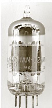
embedded in the glass base is made from an alloy which has the same coefficient of expansion as the glass to prevent the vacuum of the tube being compromised. As the tube heats up the glass and metal pins expand and if they expand at different rates the seal between them will open up allowing air to enter the tube. Having the pins come through the glass was a real technological achievement and significantly simplified the manufacturing process.
